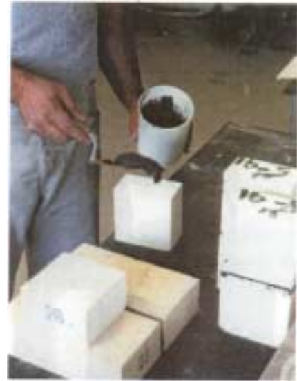
15: Joint, strength tests. Trowel application.
