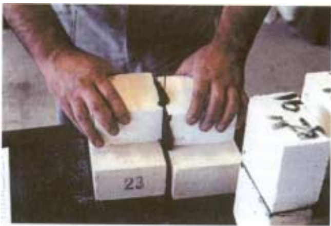
16: I.F.B. 's bonded together with regulated joint thickness (note 2 wires).
